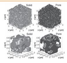
The porous electrode of a polymer electrolyte fuel cell is imaged using X-ray computed tomography with a resolution of 50 nm, achieved using Zernike phase contrast. The three-dimensional reconstructions are validated against transmission electron microscopy and mercury intrusion porosimetry.
