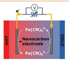
Nanocarbon-based thermocells involving aqueous potassium ferro/ferricyanide electrolyte are investigated as an alternative to conventional thermoelectrics for thermal energy harvesting. The nanocarbon thermocell may become an attractive alternative for harvesting low-grade heat, given its simple design, direct thermal to electric energy conversion, continuous operation, low expected maintenance, and zero carbon emission.
