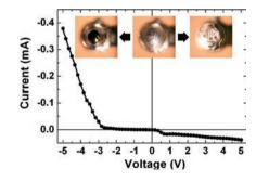
A soft-matter diode composed of hydrogel and a gallium-based liquid metal is reported. The thickness of an insulating oxide skin on the liquid metal electrode depends on the direction of the bias and can be harnessed to produce ionic current rectification. The rectification behavior is a function of the environment in the hydrogel including the local pH and the ionic conductivity. Such principles could be used in new generations of soft and biocompatible devices.
