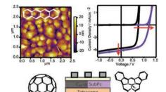
High-efficiency fullerene-free single heterojunction organic photovoltaic (OPV) devices are achieved via the replacement of  $C_{60}$  with the typical "donor" material boron subphthalocyanine chloride (SubPc). Devices containing SubPc achieve a 60% increase in open-circuit voltage, one of the largest to date for single heterojunction devices, allowing for an increase in cell efficiency from 1.8% to 2.9%.
