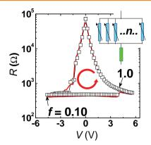
Multi-state resistance-switching thin film memory is modeled for the first time using a parallel circuit model, which successfully accounts for all the resistance-switching features as function of voltage and time, thus providing a unifying framework to predict fast data write/rewrite and memory retention.
