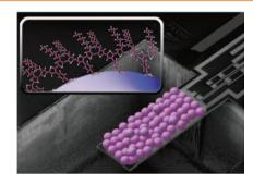
The surface of  $TiO_2$  porous films is modified by terthiophene monomers and the adsorbed monomers are polymerized at the surface of  $TiO_2$  nanoparticles. The  $TiO_2$  porous films covered with polythiophene layers work as highly sensitive sensing interfaces to provide two output signals for weight and resistance changes during exposure to vapors of volatile organic compounds.
