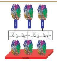
A hybrid integrated system constituting a hematite nanoparticulate film and a light-harvesting protein (C-phycocyanin) is developed. The system shows a two-fold increase in the photocurrent in comparison to the pristine hematite film. The system also shows enhanced efficiency in the visible region due to the light-harvesting action of the protein.
